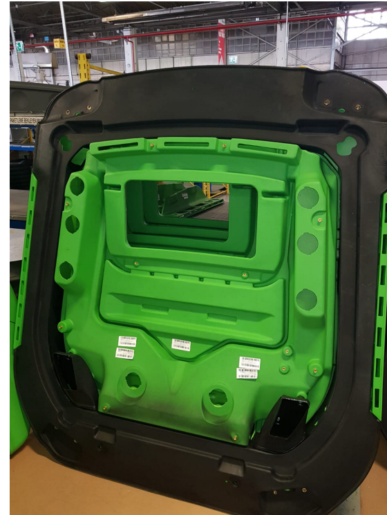
Automotive industry, truck roof, with in mould spray coating in black
