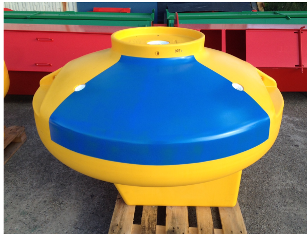
Figure shows coating done on a PE buoy with solvent based ink.
