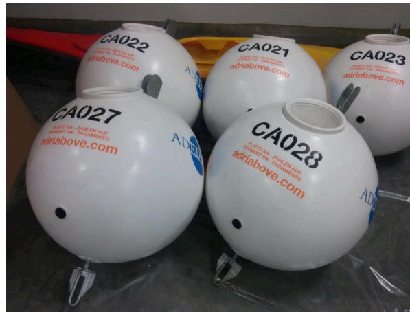
Multi-colour graphic on a PE buoy with stencil and gloss roller
